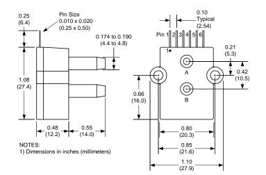
pin 1: N/C pin 2: +V supply pin 3: +Voutput pin 4: -Vsupply pin 5: -Voutput
